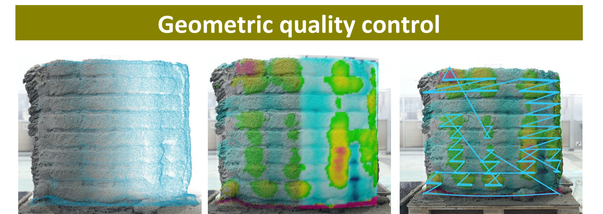
Fig. 5: Deviation of as-planned & as-built with path planning for surface improvement
