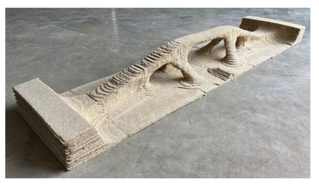
Printed structure after stiffness shape-topology and mass shape optimization
