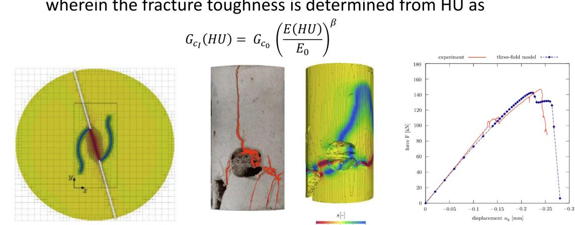
Virtual shear disk experiment CT scan to limit load for a core sample of rock
