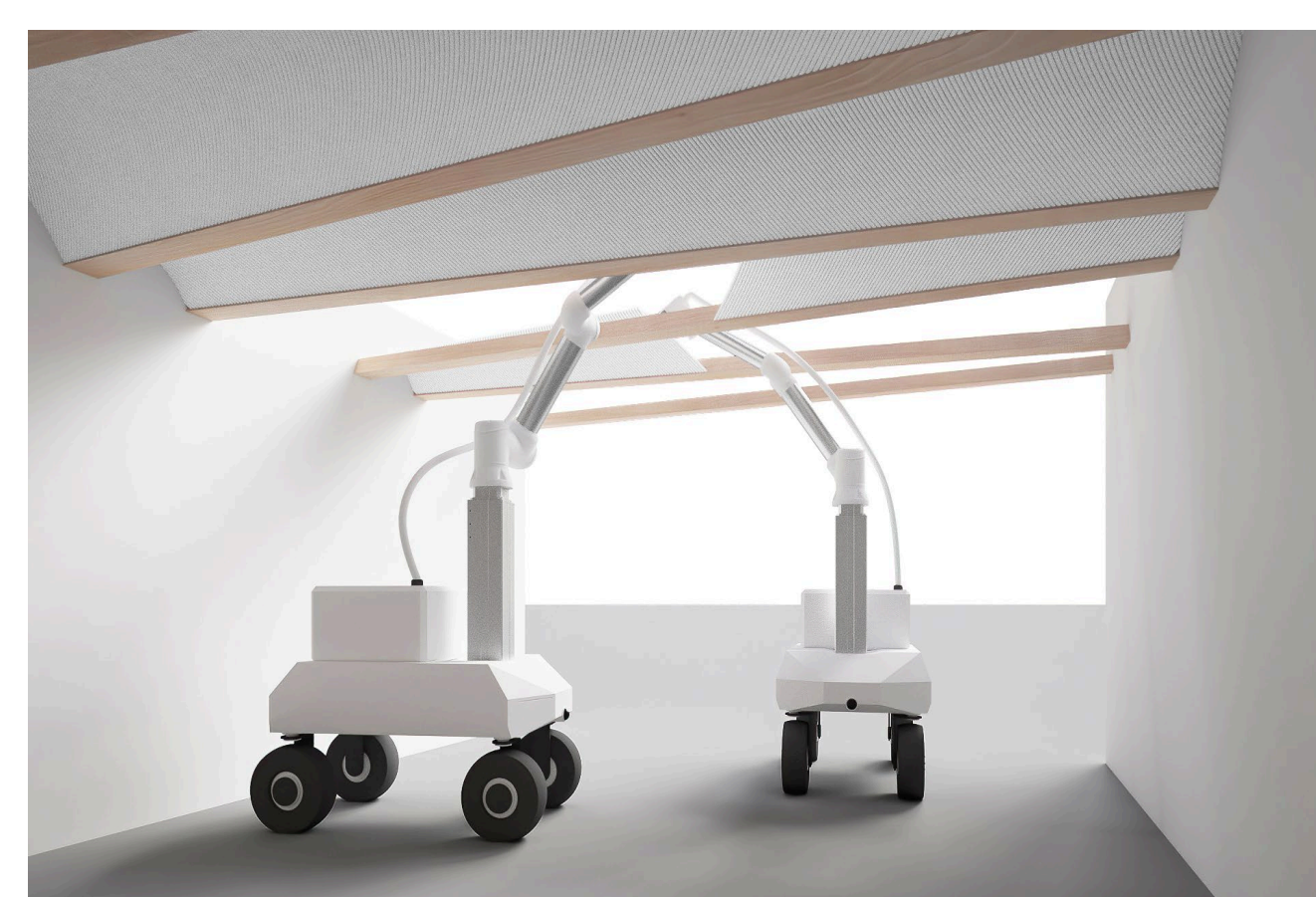
Figure 11: Multi-AMR extrusion-based AM on longitudinal beams for the creation of a vaulted ceiling geometry.
