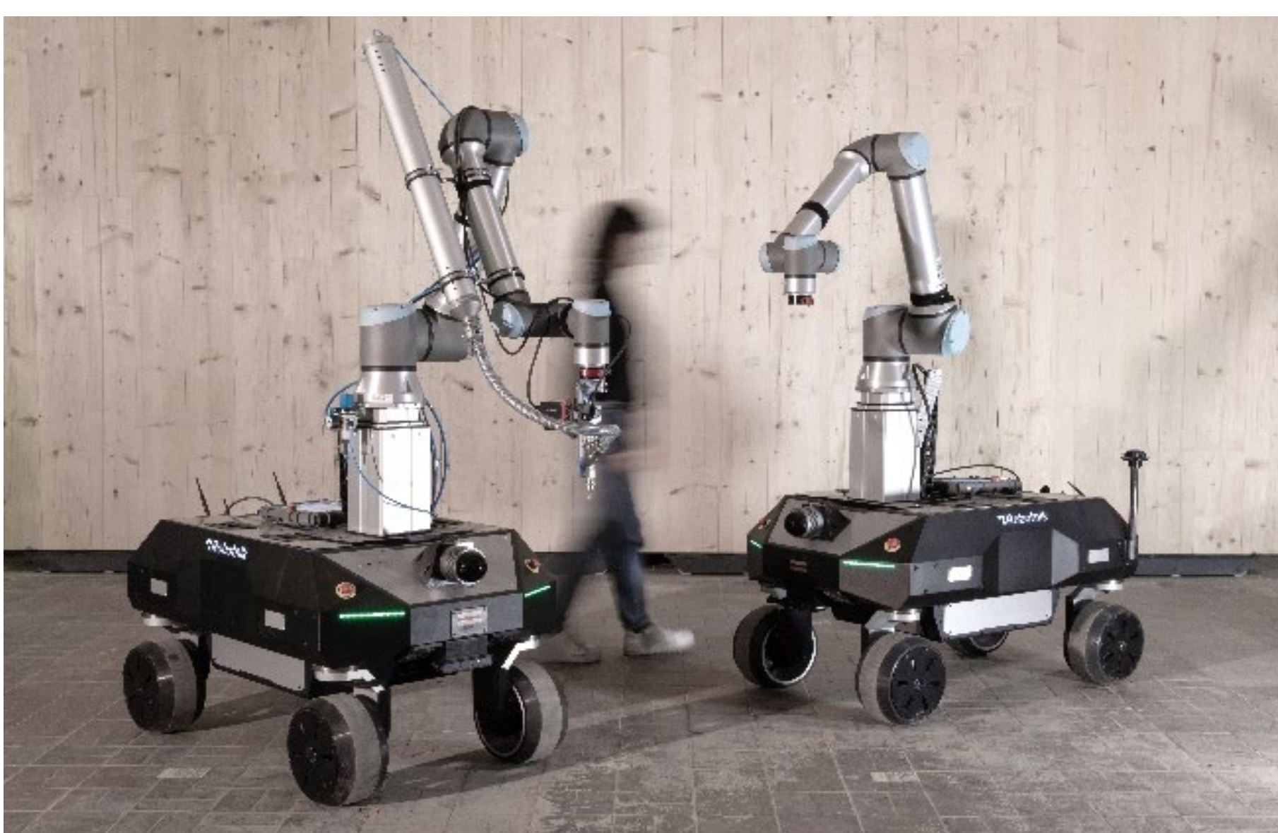
Figure 1: Two mobile robotic systems, left system is equipped with clay extrusion setup.
