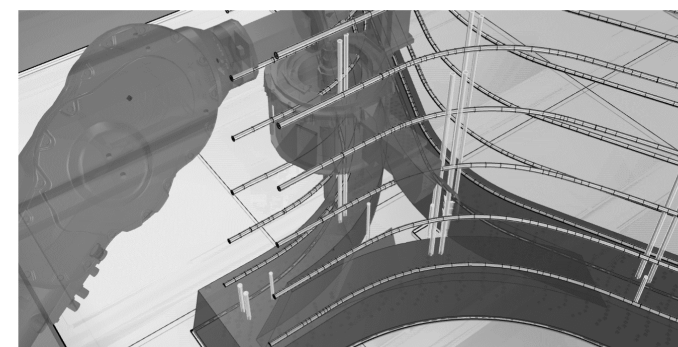
Fig. 2: Additional path parameters for robot dynamics, multi-material printing, and object integration such as rebar
