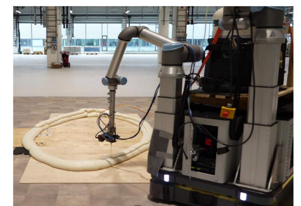
Fig. 6: Contour following to enable print-while driving
