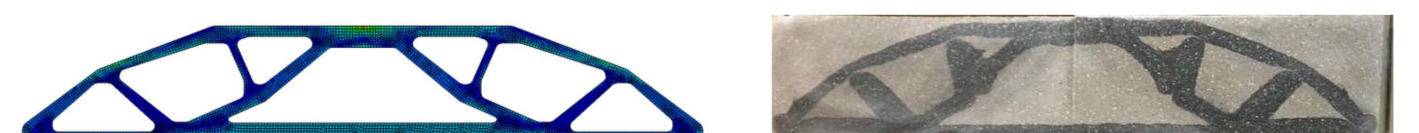
Fig. 5: Inspiration (left), Source: Deese et al. (2014); and fabrication (right) of a Concrete in Concrete (CiC)-demonstrator
