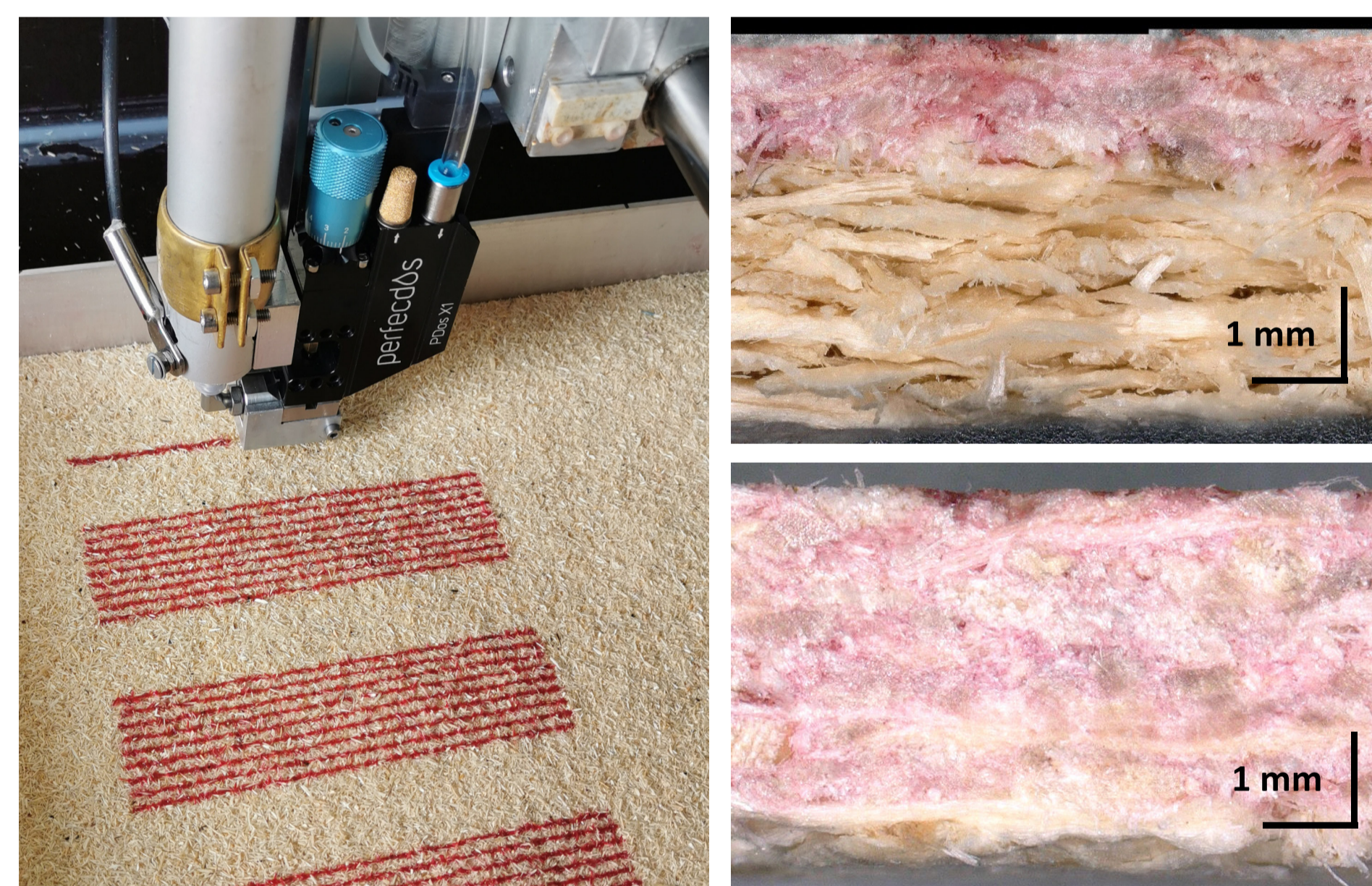
Figures Particle Scattering: Left: layer of scattered wood particles Top right: close up picture of wood particles Bottom right: wood particles in fibre shape analysis Figures Adhesive Dispensing: Left: adhesive dispensing with heated nozzle Top right: not fully intruded adhesive in particle layer Bottom right: fully intruded particle layer Figures Heat Pressing: Left: panel fabrication machine with heat press in the back Top right: the influence of pressing force on part density and flexural strength Bottom right: the influence of pressing duration on part density and flexural strength Figures Unpacking and Lamination: Top left: cleaning of the panels by hand Top right: orientation of panels for manual lamination Bottom left: cleaning of a panel with brush roller machine Bottom right: automated dispensing of adhesive for lamination
