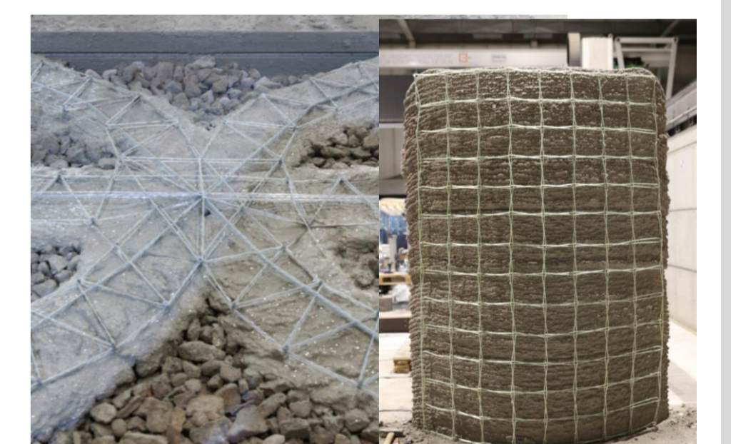
Fig. 10: Example for Pin Grid Winding
