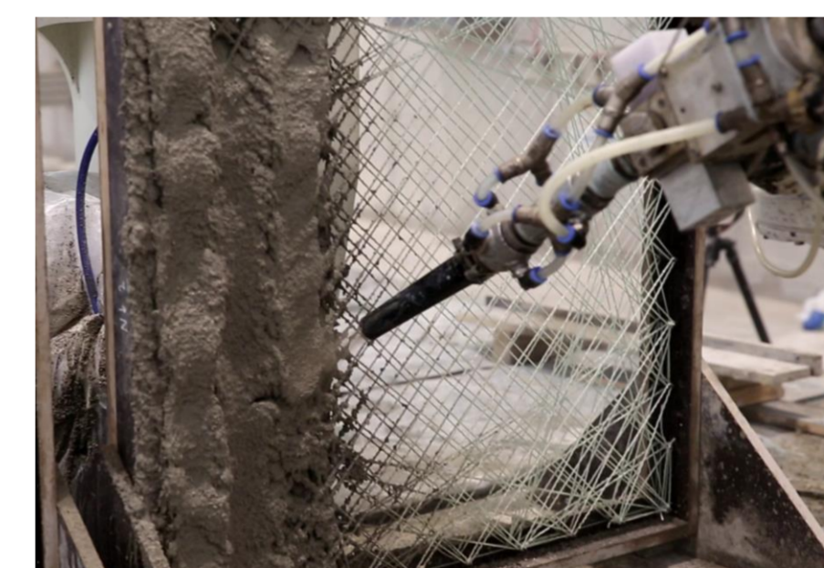
Fig. 9: Example for Frame Winding
