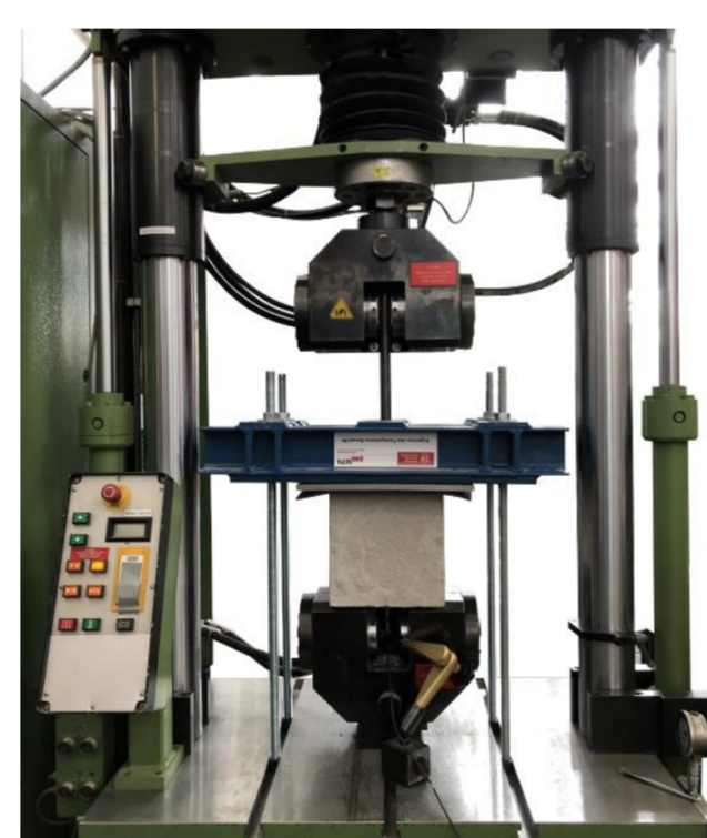
Fig. 6: Test setup for pull-out testing
