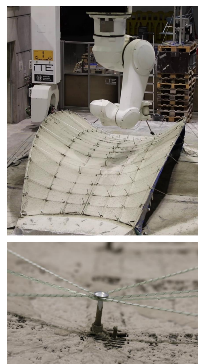
Fig. 11: Robotic fibre integration in large scale fabrication
