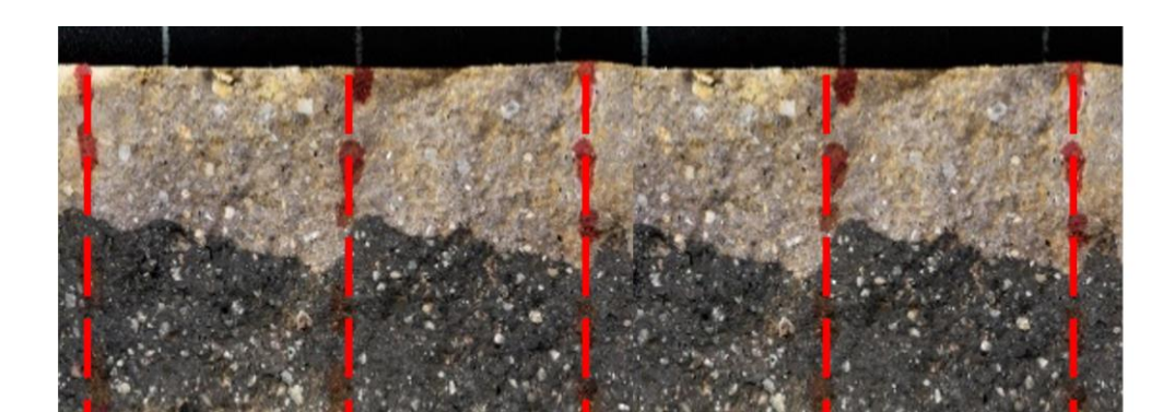
Fig 4: Chloride migration for SC3DP specimen, Credit: IBMB, TUBS
