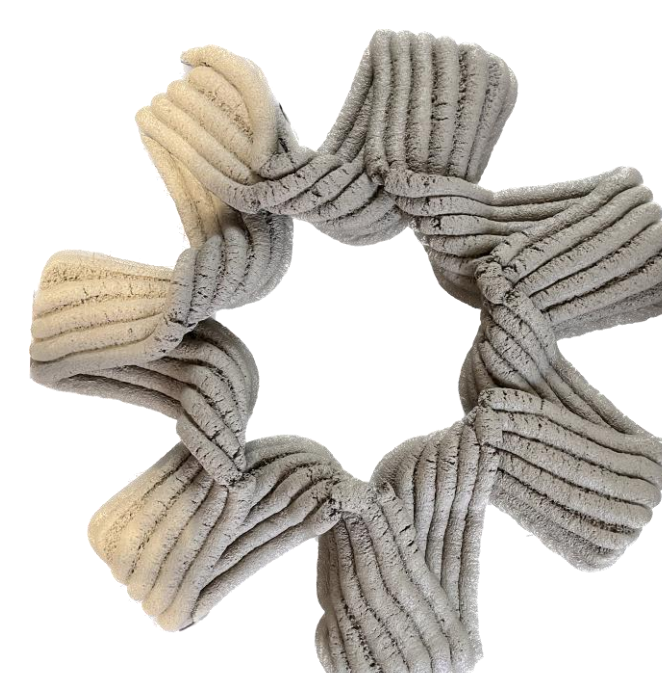
Fig. 7: Collapsed 7 tip column due to overhang tests
