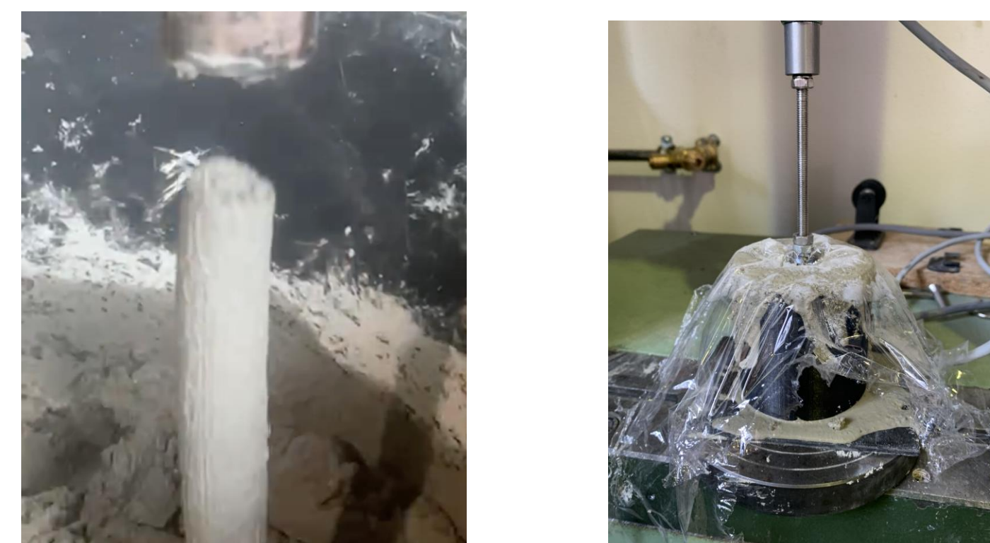
Fig. 6: Slug test with GRES V1.3 (left), slow penetration test (right)
