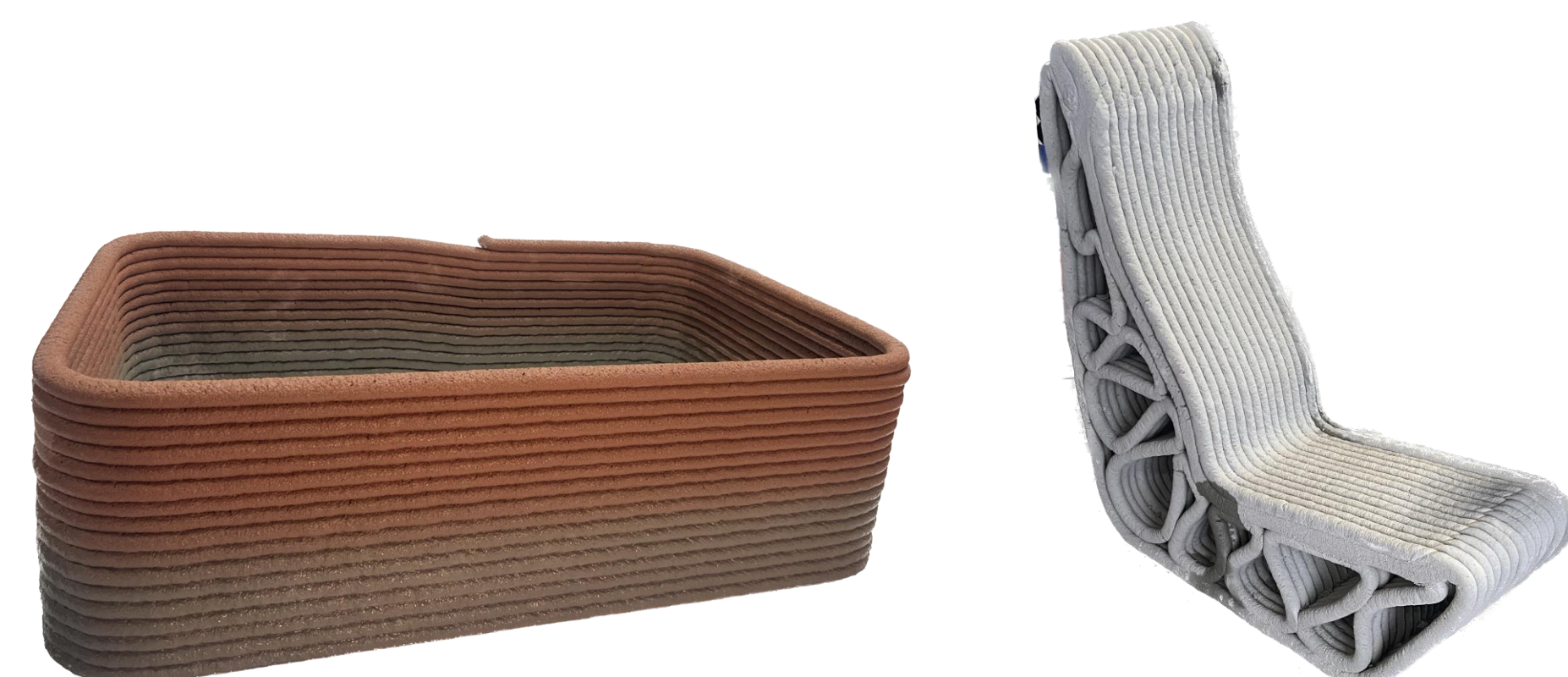
Fig. 3: First graded wall section produced by GRES V2 bottom layers SBM top layers LWM
