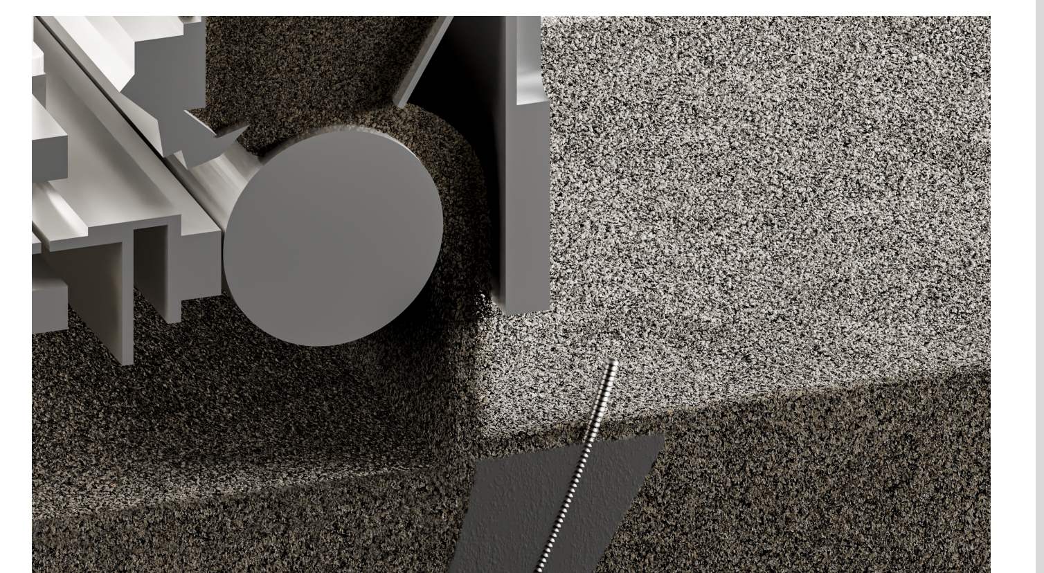
Fig. 4: Collision between a scattering roller and a protruding steel reinforcement
