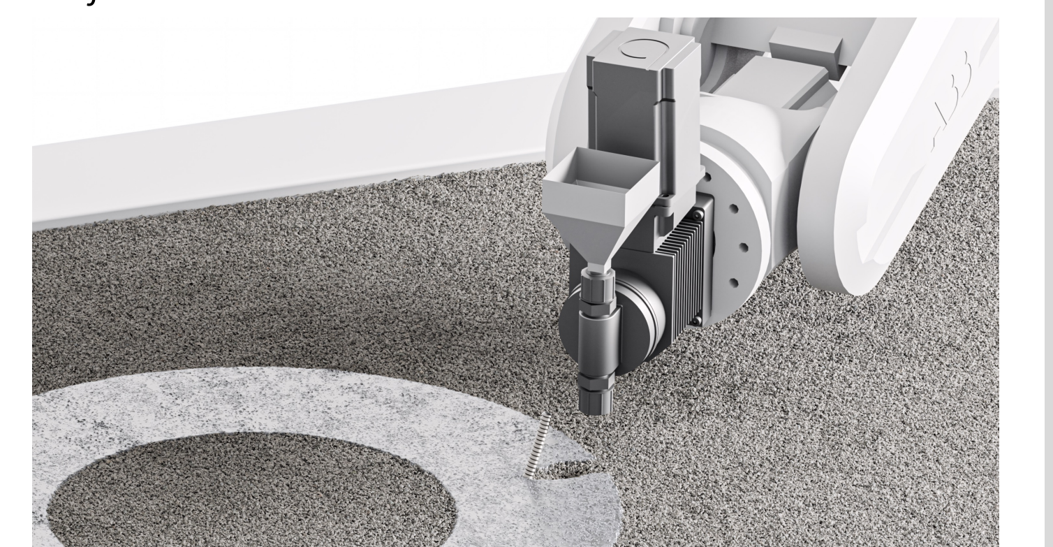
Fig. 5: Schematic illustration of a machine extension to fill up shadowed areas
